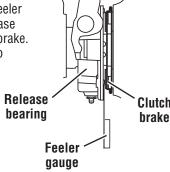
5 Slowly let up on the pedal and check the pedal position at the moment the gauge can be removed.
