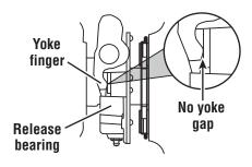
2 Fully press the pedal up to 5 times to move the release bearing slightly closer to the transmission and gain free-play in the cab.
