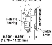
2 To change bearing position, you must internally adjust the clutch. Push pedal and hold pedal down when adjusting. Follow instructions for Kwik-Adjust or Value Clutches.
