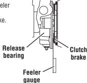
4 Slowly let up on the pedal and check the pedal position at the moment the gauge can be removed.
