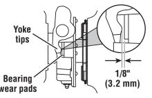
6 To change the yoke finger and bearing wear pads clearance, adjust the upper pedal stop to raise or lower the pedal in the cab.
